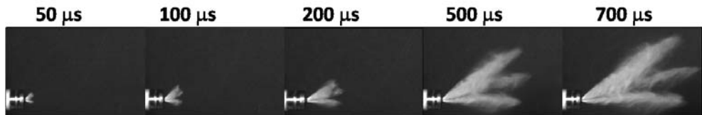
Fig. 5. Sequence of sprays from Injector #2 taken at different time from the SOI at P_{inj} = 10 \text{ MPa} , m_t = 50 \text{ mg} .
