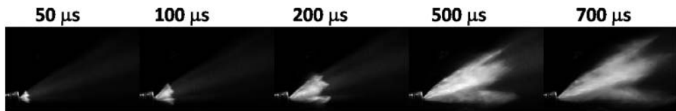
Fig. 4. Sequence of sprays from Injector #1 taken at different time from the SOI at P_{inj} = 10 \text{ MPa} , m_t = 50 \text{ mg} .
